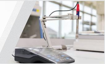
One of the electrodes is sensitive to hydrogen ions (usually a glass electrode) and the other is the reference electrode (e.g. a silver chloride electrode). They are often combined as one compact electrode together with a temperature probe.
