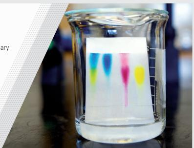
The separation is based on adsorption, partition, ion-exchange or on a combination of these mechanisms and is carried out by migration of solutes (solutions of analytes) in a solvent or a suitable mixture of solvents (mobile phase or eluent) through the thin-layer (stationary phase).
