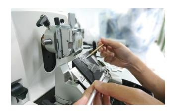
**Paraffin** is one of the most used products in laboratories of Anatomic Pathology. The paraffin blocks are placed on a device that uses an extremely sharp knife (a **microtome**) to obtain very thin pieces of tissue.
