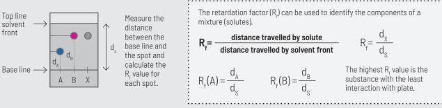
Thin-layer chromatography can be used to monitor the progress of a reaction, identify compounds present in a given mixture, and determine the purity of a substance. Specific examples of these applications include: analysis of ceramides and fatty acids, detection of pesticides or insecticides in food and water, analysis of the dye composition of fibers in forensics, assaying the radiochemical purity of radiopharmaceuticals, or identification of medicinal plants and their components.
