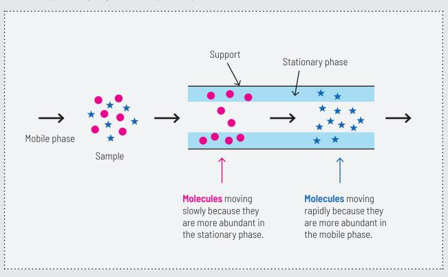
The separation may be based on adsorption, mass distribution (partition), ion-exchange, etc. or may be based on differences in the physico-chemical properties of the molecules such as size, mass, volume, etc.
