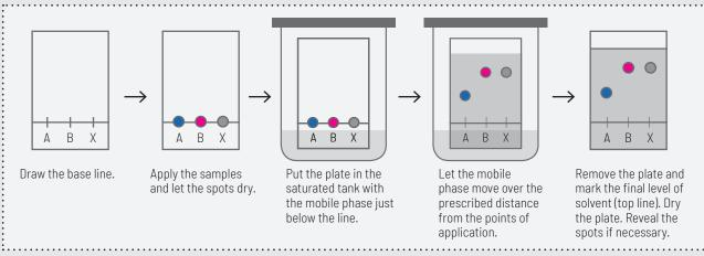
After the experiment, the spots are visualized. Often this can be done by simply projecting ultraviolet light onto the sheet; the sheets are treated with a phosphor, and dark spots appear on the sheet where compounds absorb the light that strikes a certain area. Specific reagents can also be used to visualize spots.
